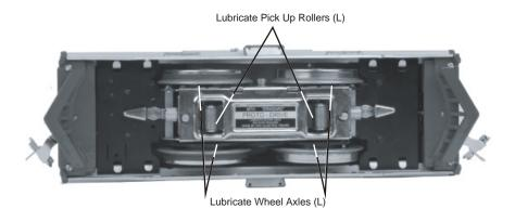
Lubrication Points on the Locomotive
