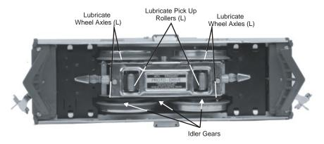
The locomotive utilizes a direct drive motor that should not need direct lubrication. However, it will be necessary to lubricate the idler gears located on the inside of the drive wheels.
