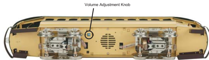
Figure 2: Manual Proto-Sound 2.0 Volume Adjustment
