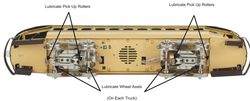
Figure 1. Lubrication Points on the Trolley
