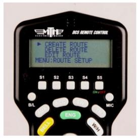
• Name the Route: Using the thumbwheel, scroll to each letter in the Route's name and press the thumbwheel to add that letter, number, or symbol to the Route name. Use the "<" character to remove an erroneous character and, when the name is complete, use the "D" character at the right end of line 3 to end the name. A Route Name may be up to 16 characters long.
