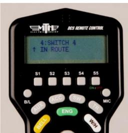
• End the Route: When you've added all the switches to the route, press soft key S4, "DONE", to end building the Route. Press MENU twice to exit the DCS Menu system.
