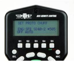
**NOTE** that the LABOR REV UP/DRIFT REV DN rocker switch on the DCS handheld *overrides this* Sound menu setting. If you use the rocker switch for a particular engine, the Proto Chuff setting on that engine will automatically be set to OFF.
