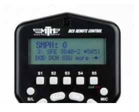
and a variety of sounds the engine will make while idling. To activate any sound, simply scroll to it and press the thumbwheel. The sound will play and you will be returned to the soft key list. When you're done playing sounds, press the ENG key to return to the Engine screen.
