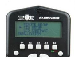
**Scroll and select SUPER TIU:** scroll to SUPER TIU and press the thumbwheel to enter Super TIU setup.
