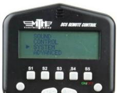
**Scroll and select TIU SETUP:** scroll to TIU SETUP and press on the thumbwheel to select DCS Setup.
