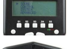
**Scroll and select SYSTEM:** scroll the thumbwheel to SYSTEM and press on the thumbwheel to select the System menu.
