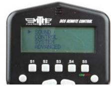
**Scroll and select ADVANCED:** scroll the thumbwheel to ADVANCED and press the thumbwheel to select the Advanced menu.
