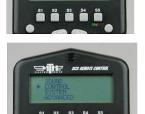
**3. Scroll and select ACC or DEC:** scroll to ACC or DEC and press the thumbwheel to adjust acceleration or deceleration
