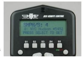
light load, and higher settings will cause the engine to speed up and slow down much faster. You can even change these settings while the engine is rolling down the rails!
