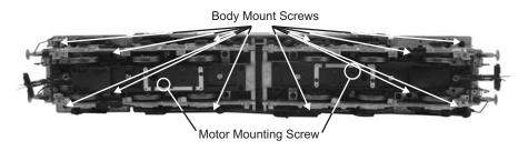
Figure 11: Body Removal Screw Locations and Motor Mounting Screws
