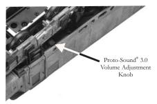
Figure 10: Manually Adjusting the Volume
